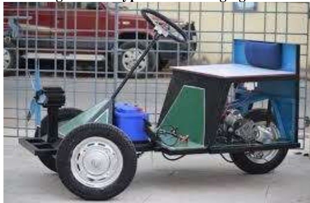
Fig-1: Prototype of Self-charging Car.
