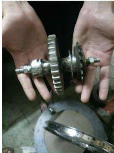
Fig.2: Spur Gear mounted on the hub.
