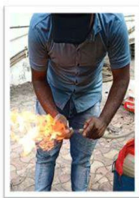
Fig. 3: burning of extracted methane gas
