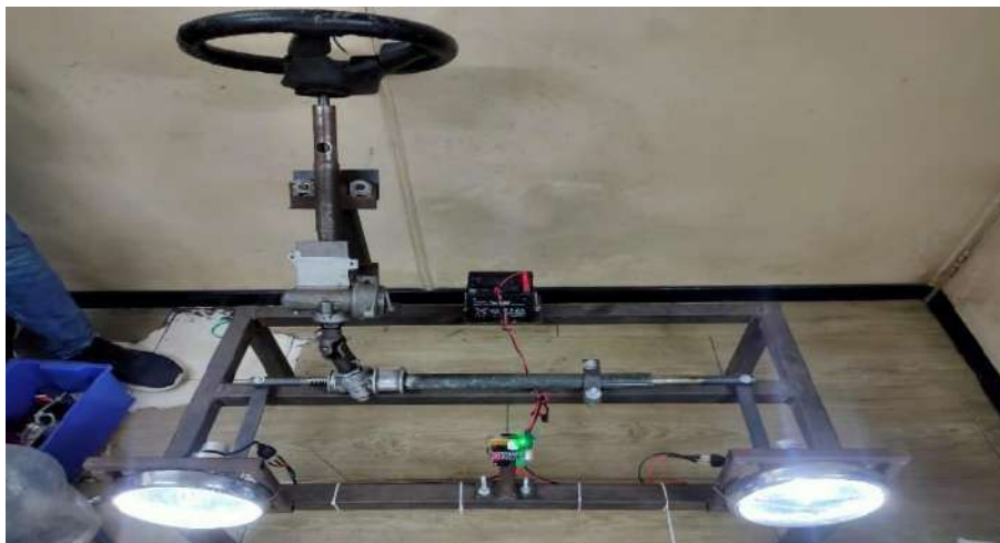
Figure 2: Final Assembly Model of the Adaptive Headlight System
