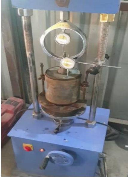
Fig. 3 CBR test construction
