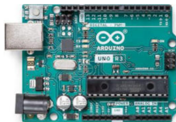
Fig.2: A typical Aurdino UNO microcontroller
