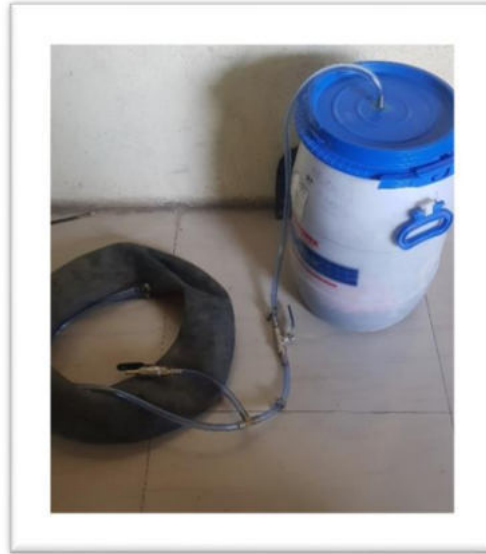
Fig.1 Mini Biogas plant developed
