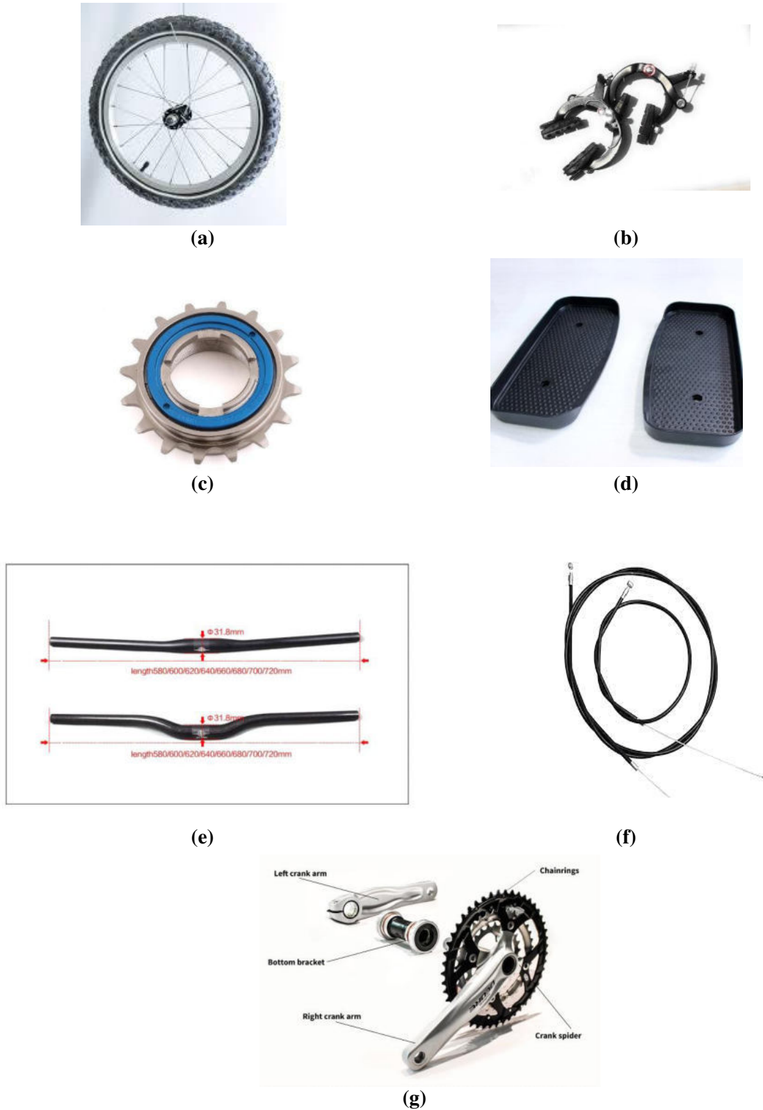
Figure 2. Parts Details (a) Wheel (b) Brake (c) Freewheel (d) Large Pedals (e) Handle Bar (f) Brake Cable (g) Crank Set
