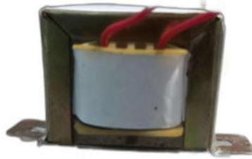
FIGURE 5: POTENTIAL TRANSFORMER ATmega328
