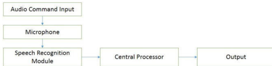
Figure 3: Speech Recognition Block Diagram
