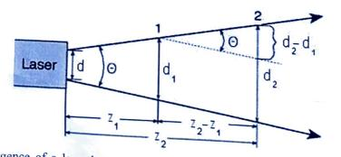
The divergence of a laser beam can be calculated if the beam diameter  $d_1$  and  $d_2$  at two separate distances are known. Let  $z_1$  and  $z_2$  are the distances along the laser axis, from the end of the laser to points "1" and "2".
