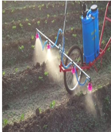
Figure 2: Working of Agrochemical Sprayer
