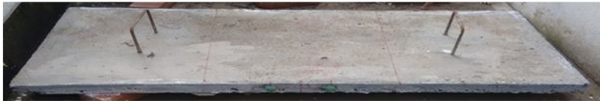
Marking of Demec Gauge Pellets
