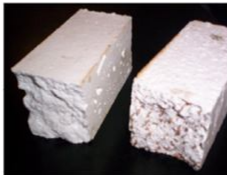
Fig. 1 – Gypsum plasters with cellulose fibres and cork
