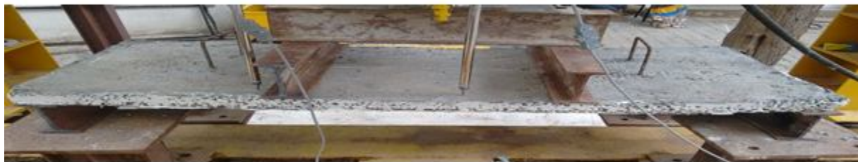
LVDT at Center and support
