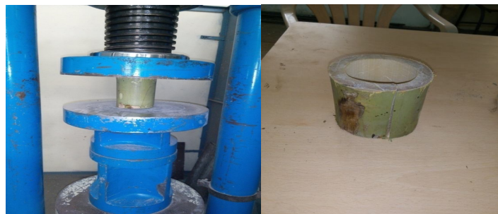
Fig.2 Compression test setup and failure pattern of bamboo sample
